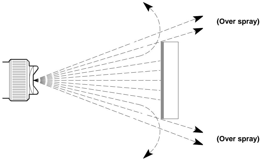
**Efficiency = Amount on target vs. Amount sprayed**
