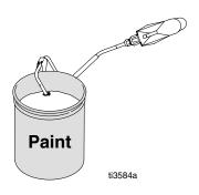
4.Place roller frame in paint pail. Be sure the holes in the frame are facing inside the paint pail.
