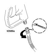
2. Connect one end of grounded fluid hose to gun. Use a wrench to tighten.
