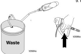
9. Place roller frame in waste pail and trigger gun. Be sure the holes of the roller frame are facing inside the pail.
