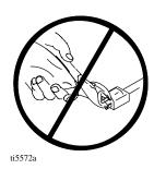
Do not use the sprayer if the electrical cord has a damaged ground prong. Only use an extension cord with an undamaged, 3–prong plug.
