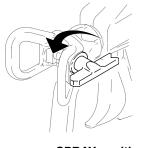
**SPRAY** position (pull trigger to paint)
