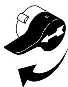
7. Turn Spray/Prime valve to SPRAY to keep storage fluid in sprayer during storage.
