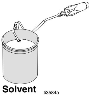
5. Place suction tube in bucket of water or compatible solvent for non-water-based materials. For flushing water-based materials, follow Zip Flush procedure, page 16.
