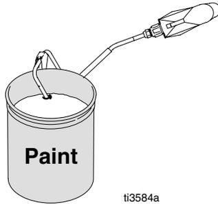
4. Place roller frame in paint pail. Be sure the holes in the frame are facing inside the paint pail.
