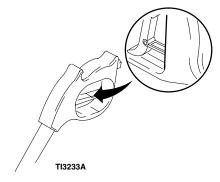
4. Adjust throttle to STOP position. Engine should turn off.
