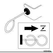
7. Pull the starter rope quickly to start the engine. Pull and return the rope until the engine starts. HINT: Placing one foot on the pressure washer as a brace provides better leverage.
