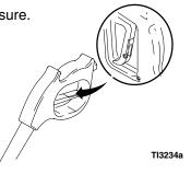
7. Remove high pressure hose from pump. Drain water from all components.
