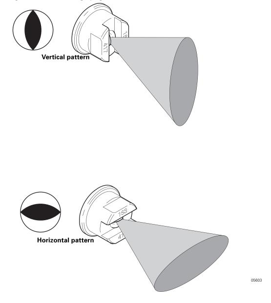
**Figure 5**: Graphic of an airless spray tip showing two views of spray patterns
