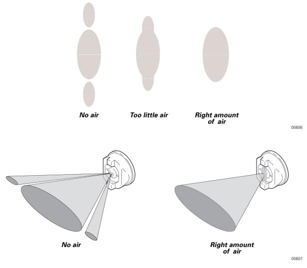
Figure 8: Air assisted airless spray patterns. Top: Typical patterns as sprayed on a surface. Bottom: How the atomizing air from an air-assisted airless gun eliminates pattern tails.
