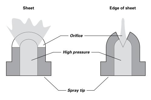
Figure 6: Airless spray tip design.
