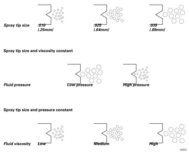
Figure 2: The relationship between the factors that affect droplet size.
