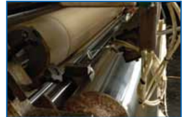
Figure 2 – Solvent-free lamination process
