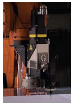
Figure 2: 20cc PGM with direct-mount applicator
