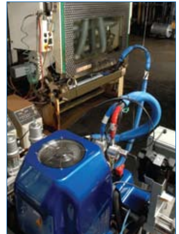
The system's MD2 Dispense Valve and static mixer are mounted to an actuator on the laminating machine that travels back and forth across the nip trough to evenly distribute the mixed material.
